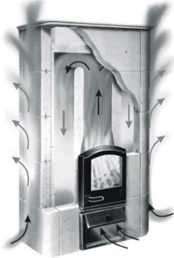
Operating principle of a masonry heater
